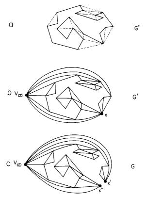
**Fig. 6.3.** The graph G in (c) is produced from a triangulation of the hull pockets (a) by connecting all hull vertices to  $v_{\infty}$  (b) and splitting some hull vertex x.
