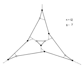
Fig. 6.19. A convex partitioning of 12 vertices that requires 7 combinatorial guards (solid dots) for domination.
