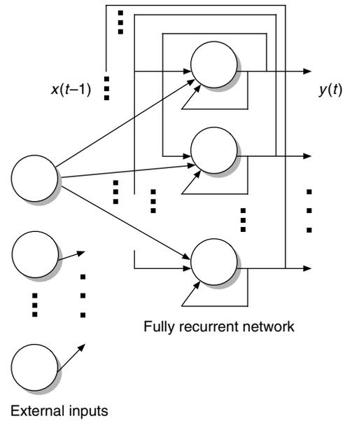
**Figure 2** A Fully Recurrent Network, with External Inputs on Left
