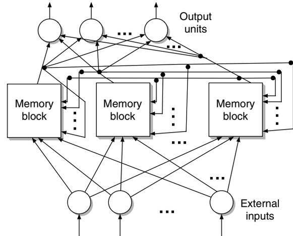
Figure 3 An LSTM Network with Recurrent Memory Blocks in the Hidden Layer Between the Input Layer and the Output Layer
