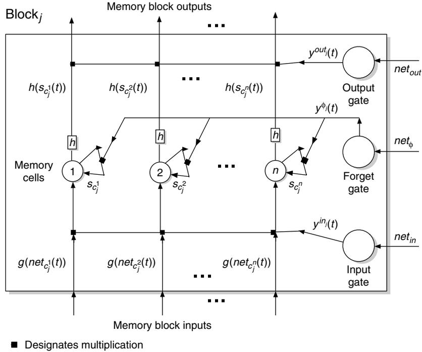
**Figure 4** An LSTM Memory Block Showing  $n$  Memory Cells and Gates Learned by Nonlinear Units Receiving Either Inputs or Values from Recurrent Connections with Other Memory Blocks
