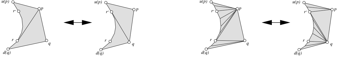
Figure 4. (i) Two points exchange in x -order. (ii) Fan triangulation of IPT(\mathcal{P}) .
